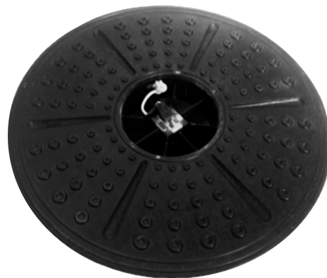
Figure 2. Phidget 3-axis Accelerometer retrofitted inside the wobble board.
