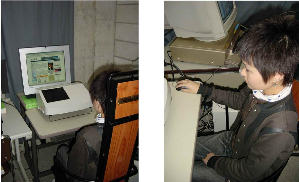
**Figure 2.** Experimental Setup. The subjects sit in front of the display without any device making physical contact with them. Eye movements are measured while each subject performs tasks by manipulating a computer mouse.
