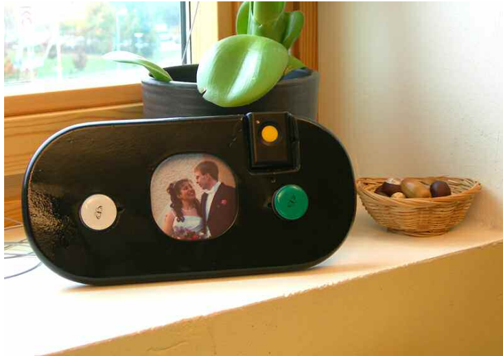
Figure 2. The photo frame remote control used with Berit's personal TV photo album.
