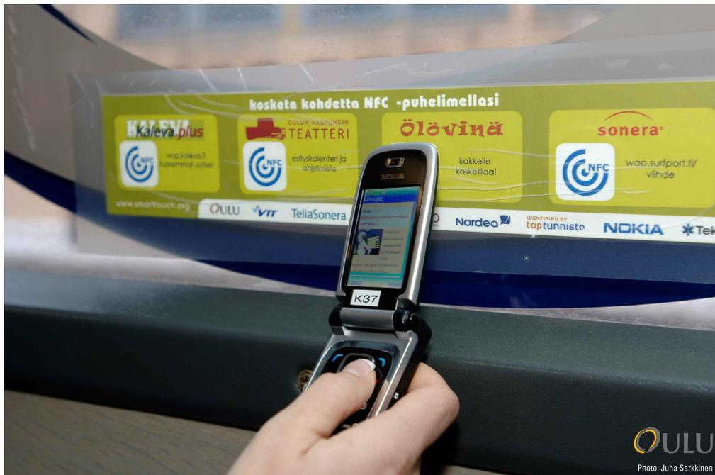
**Figure 1.** With NFC tags, users can access mobile services and content just by touching a tag placed in a physical space with their mobile phone.
