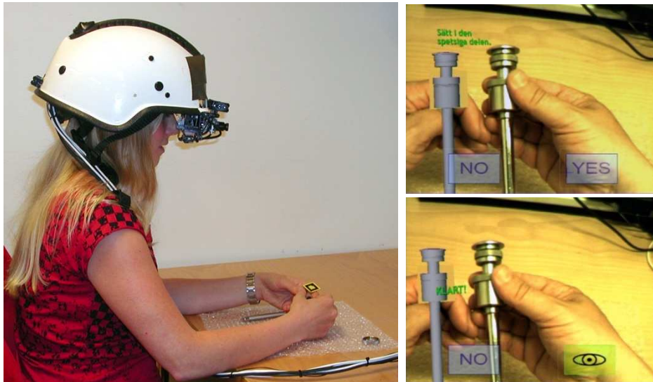
Figure 7. The gaze-controlled AR system in the second application. The images to the right show what the user sees. The “no” represents repeating an instruction (going back in the sequence), and the “yes” means going to the next step. Note that, in this setting, the interactive area is placed in the lower part of the display rather than the upper part as in the examples above.
