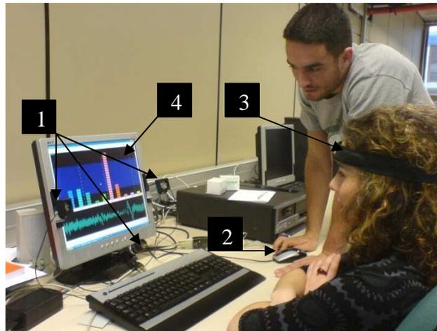
**Figure 6.** Experimental setup in Experiment 2: (1) Eye tracker. (2) Mouse. (3) Cyberlink™ headband. (4) 17-inch monitor. The display is showing the Cyberlink™ software.
