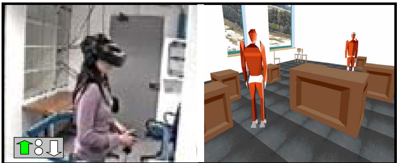
Figure 3: An AIAD, at the bottom of the screen, shows an arrow indicating that the button for the movement forward is pressed .
