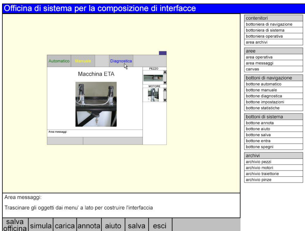
Fig. 4: A part of the application workshop has been created. The button “diagnostica” (diagnostic) is being located on the operative button panel.
